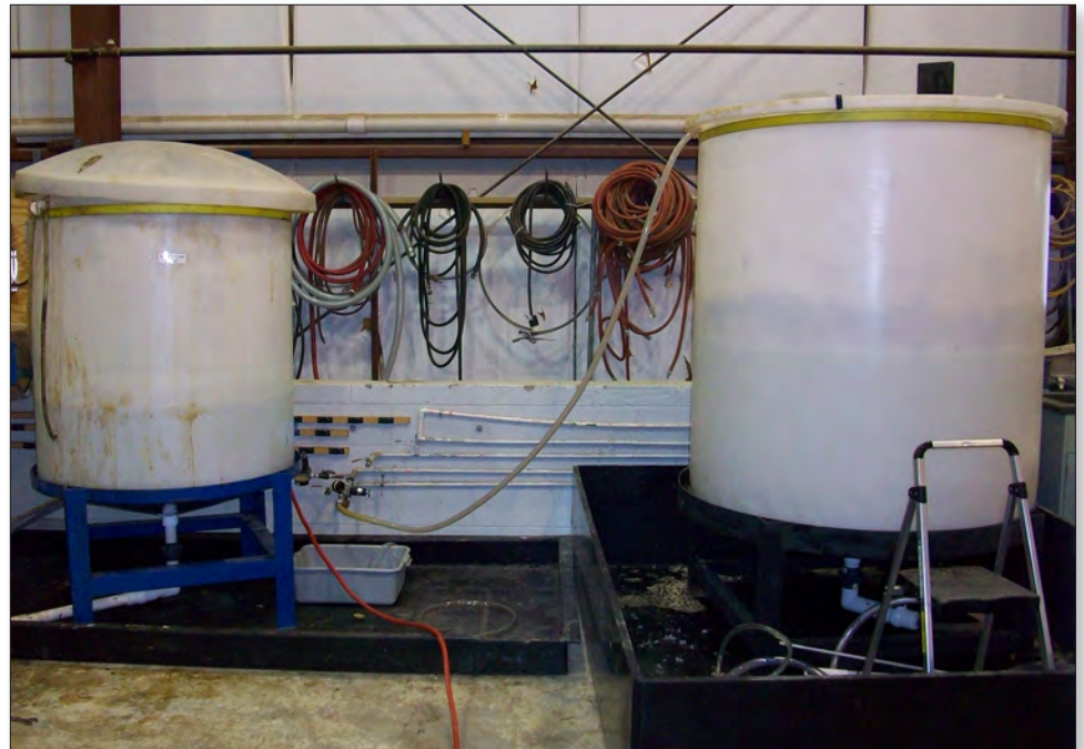
The experimental 400-gallon and 800-gallon bioreactors used to assess the chemical properties of the biopolymer produced using varied food industry waste by-products and develop production parameters for industrial scale-up. (Photo by David Roberts, PAO-ERDC)
