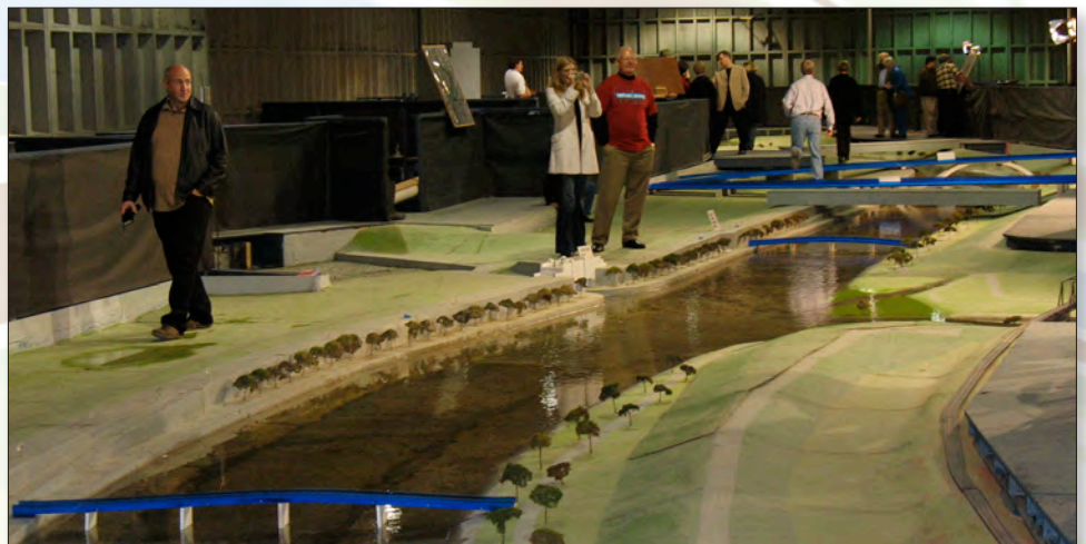
Fort Worth Central City Project- Hydraulic Scale Model (courtesy of Laura Bacigalupo, Public Information Officer, Trinity River Vision Authority)
