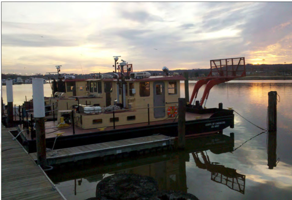
BD-5, one of Baltimore District's debris vessels in Washington, DC and the first USACE vessel to operate on B100 biodiesel (Photo by Bob Leitch, HQ USACE)
